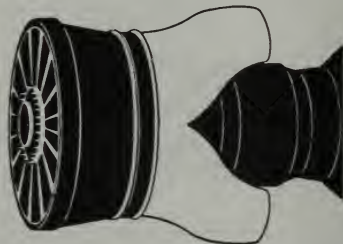
FIGURE 2-27. Bifurcated duct configuration.
